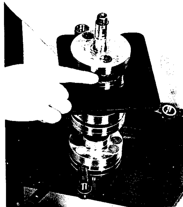
4 Place the flywheel support plate (tool S) between the flywheels of the left-hand crank assembly. (Position the support plate so that the big end of the connecting rod is at the closed end of the rod access slot in the support plate.)
